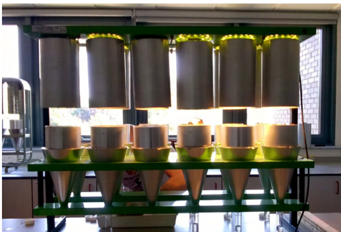
Figure 5: Burlese funnels set up to extract invertebrates from leaf litter
